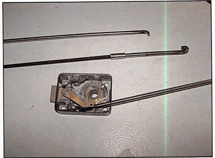
Photo 5 shows the tool in the lock made from air hardening drill rod with a screwdriver handle used to pry the lever into the drive cam gate. The bent end of the tool was sharpened parallel to the shaft of the tool. A second tool is sharpened in the opposite direction or 90 degrees to the tool used. The puller rod tool is between the lock and the second tool. Normally the puller would be used to grab the strap of the lock bolt extension either below or above the lock, depending on how the safe was produced.
